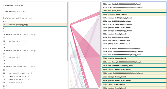
Fig. 5. An early prototype visualizing the mapping between source code and disassembly. Even in this toy example, a single line of code is dispersed across the disassembly. Early prototypes like this one also clarified the importance of the CFG in conveying structure.
